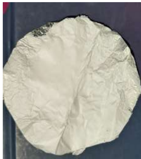
Figure 1. Electrospun PVA nanofibers obtained from a 10% (w/v) solution under an applied voltage of 20 kV and a feed rate of 900 \mu\text{L h}^{-1} .
